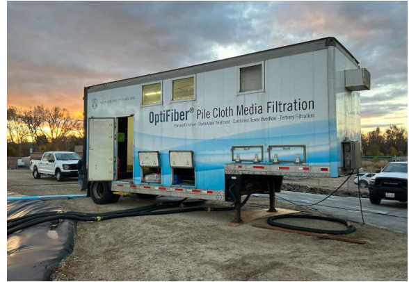
Figure 1: 2-micron cloth disc filter pilot
