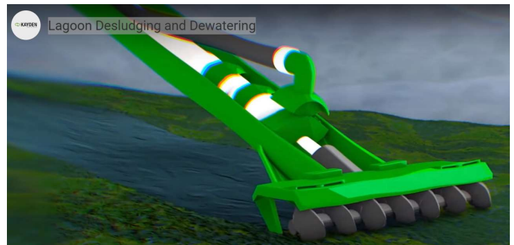
Figure 2: Dredge cutter head that removes solids
