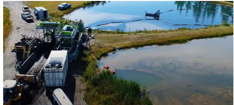
Figure 1: Mobile dewatering setup with dredge and centrifuges
